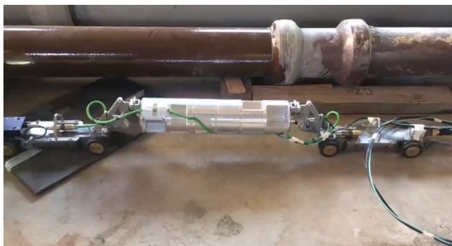
Fig. 10: Evaluation sample: 3D sensor head with multiple camera-projector modules
