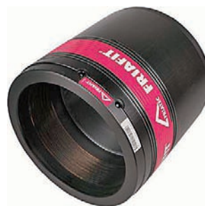
Fig. 17: Transition Coupler AMKG with integrated slip-on coupler for the direct connection of a PE-pipe with a PVC/PP pipe
