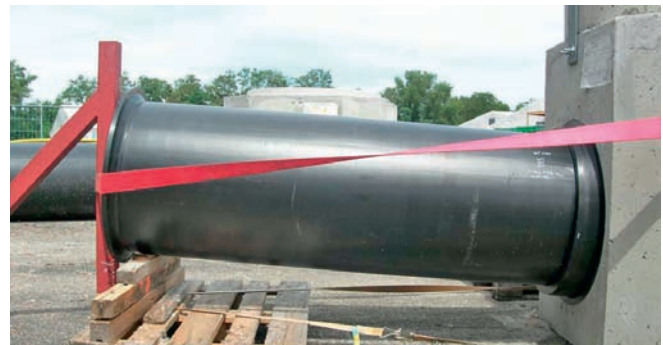
Fig. 9: Test of an inspection chamber connection d630
