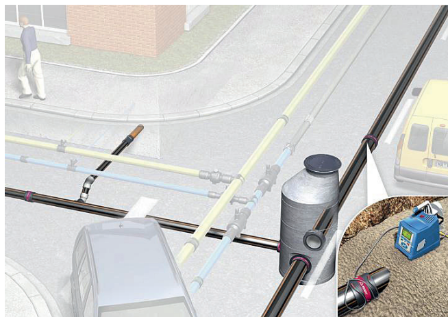
Fig. 3: Sewer infrastructure with PE pipes
